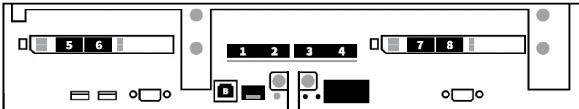
Figure 5. Recommended DGX H100 system network port connections.
