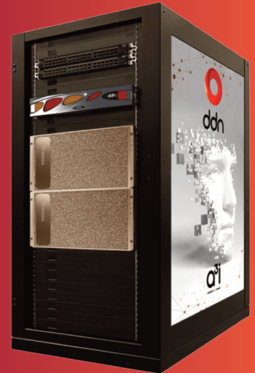
DGX SuperPOD with Two NVIDIA DGX nodes and DDN A 3 I storage
